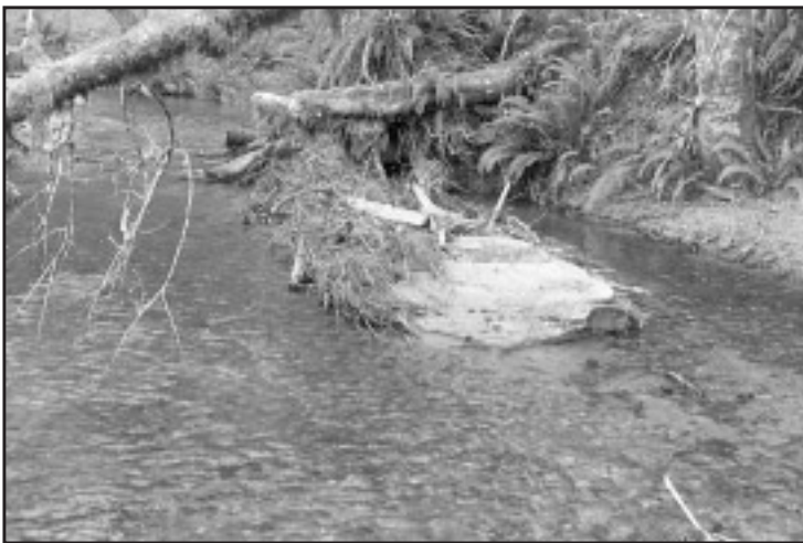
Figure 6. A four-PCT bundle tied to a root extending from the stream bank. Note the deposition of fine material after only half of the winter season had passed.
