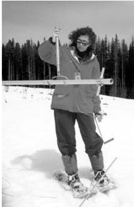
Surveys of snow depth and water content in forest and clearcuts occur regularly during late winter and early spring.
