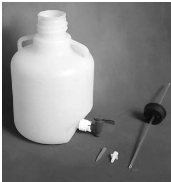
Figure 1. Materials required to construct Mariotte bottle. From left to right: 10-L carboy, pipette tip, Quick Disconnect Connector, rubber stopper with Plexiglas tube inserted.
