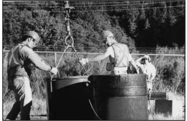
Figure 2. Operating the self-dumping buckets that were fabricated for the helicopter.
