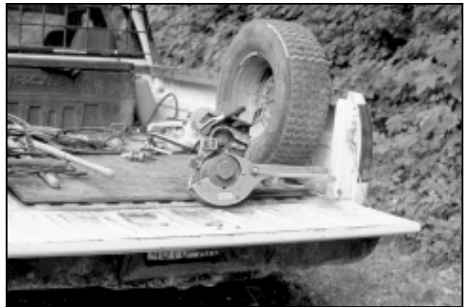
Figure 3. The Zollern winch without the line cage in the back of a pickup truck.
