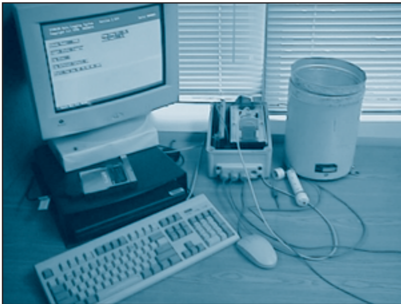
Figure 3. This is a photo of the equipment installed at the two Ministry of Forests sites in the Hesquiatic Basin. To ensure the accuracy of the data, the installations are periodically replaced with spare units and brought back to the office where the sensors are calibrated.
